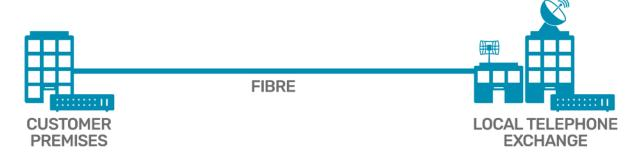
Fibre is the "Rolls Royce" internet access solution and requires the provider to deliver a piece of dedicated fibre into the business premises from the local exchange. Once a piece of fibre has been provisioned into the business premises then the potential for internet bandwidth is limitless.
